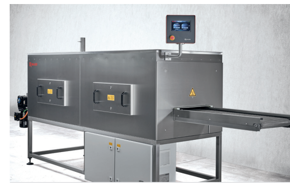
Conveyor oven for hardening of electronic components – two heating circuits, exhaust air controls and a chain transport system are integrated.
